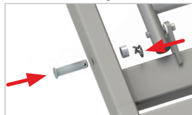
8.2.5 Clevis pin, spacer, and R clip fitting
